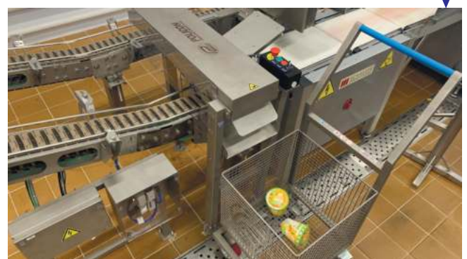
Rejection of products without a digital code by a broker
